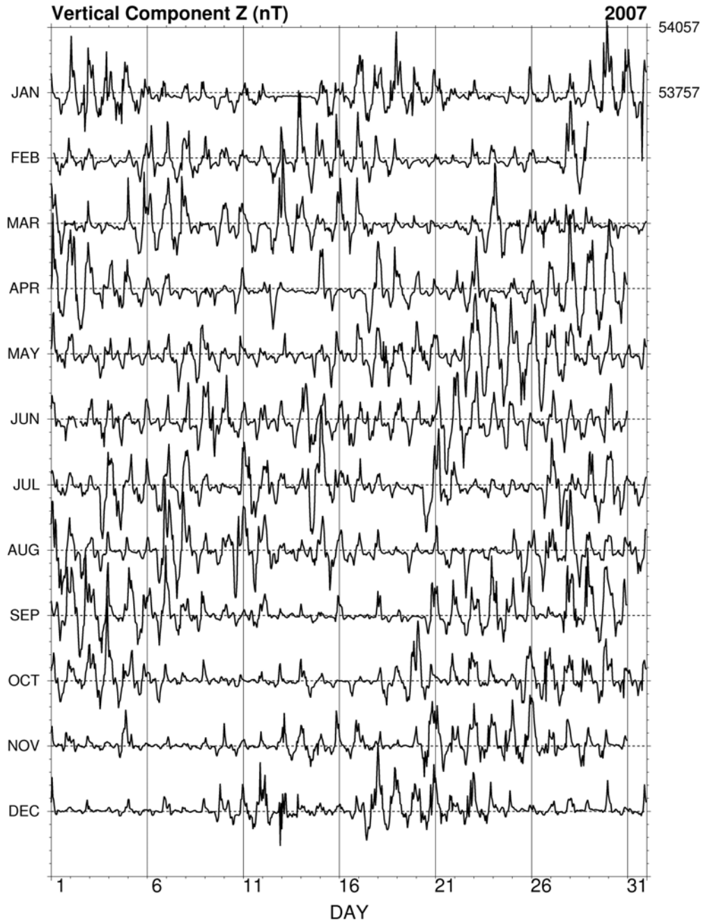
Fig. 31. Hourly mean data plot of Z component for Hornsund.
