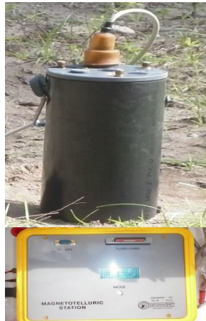
Fig. 3.9: Two MS-27 variometers are in field stations
