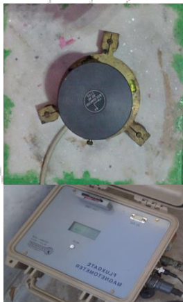
Fig. 3.4: GEOMAG-02M variometer as secondary system in HYB
