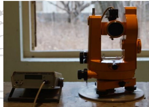
Fig 3.12: THEO-020A & GEOMAG-03 absolute magnetometer for field stations
