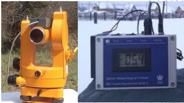
Fig. 3.11: THEO-020A absolute magnetometer for field stations
