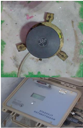
Fig. 3.8: Four GEOMAG-02M variometers are in field stations
