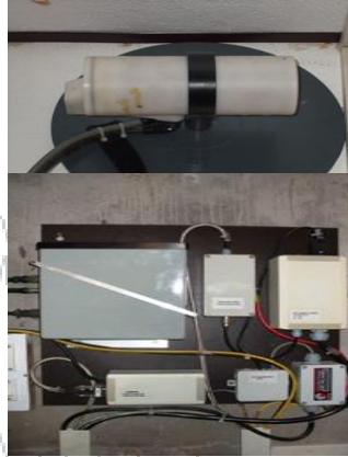
Fig.3.2: Two GSM90 Overhauser are total field magnetometers as primary systems at HYB & CPL
