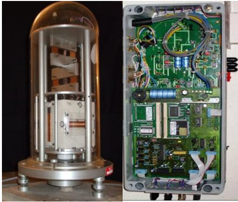
Fig.3.1: DFM variometer systems two, one in HYB & CPL as primary variometer system
