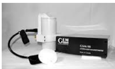
Fig. 3.7: GSM90 Overhauser total field magnetometer for calibration both at HYB & CPL
