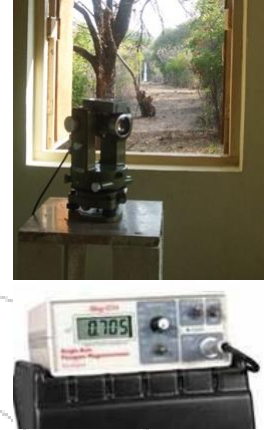
Fig.3.3: Two WILD-T DI-flux magnetometers at HYB & CPL
