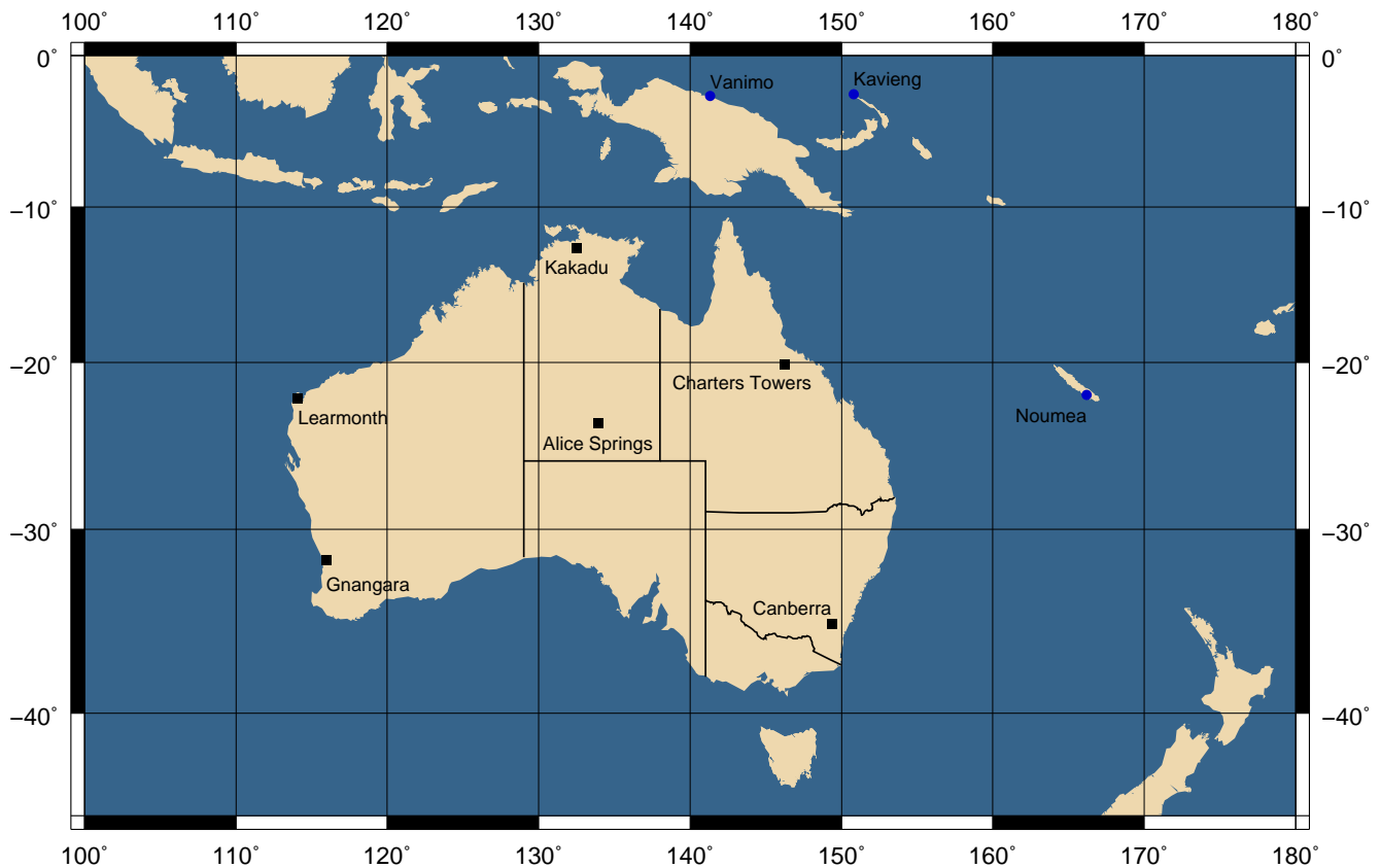
Figure 10.1. Repeat stations occupied in 2007 (blue dots) and the Australian magnetic observatory network (black squares).
